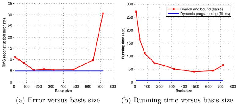
Fig. 4: While the basis size in [1] is not critical, an incorrect choice still adversely affects the reconstruction (a). Filter prior obtains a slightly better reconstruction than the best basis reconstruction. The filter objective could be minimised using branch and bound but the reconstruction will be identical. The running time of the branch and bound method varies with the basis size (b). Results were averaged over  $8 \times 800$ -frame sequences.
