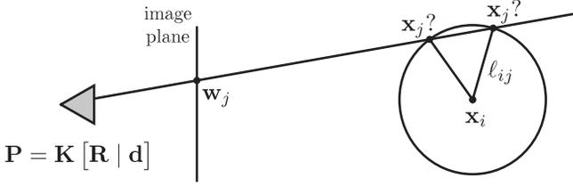
Fig. 2: With known camera  $\mathbf{P}$ , parent point  $\mathbf{x}_i$ , edge length  $\ell_{ij}$  and 2D projection  $\mathbf{w}_j$ , there is a two-fold ambiguity over the position of the endpoint  $\mathbf{x}_j$  in each frame. This is true of full perspective and affine cameras.
